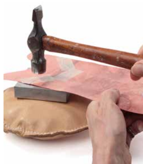
Scoring with a Hammer and Block
