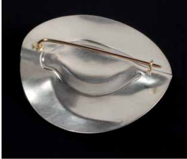
A gold pin and catch were soldered onto this silver score-folded form to create a brooch.
