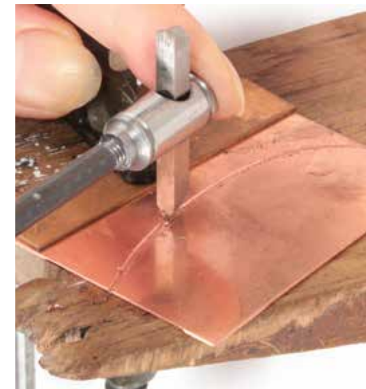
Using a Scoring Tool to Cut a Curved Score
