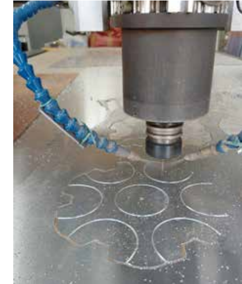
Scoring with a Computer Numeric Controlled (CNC) Router
