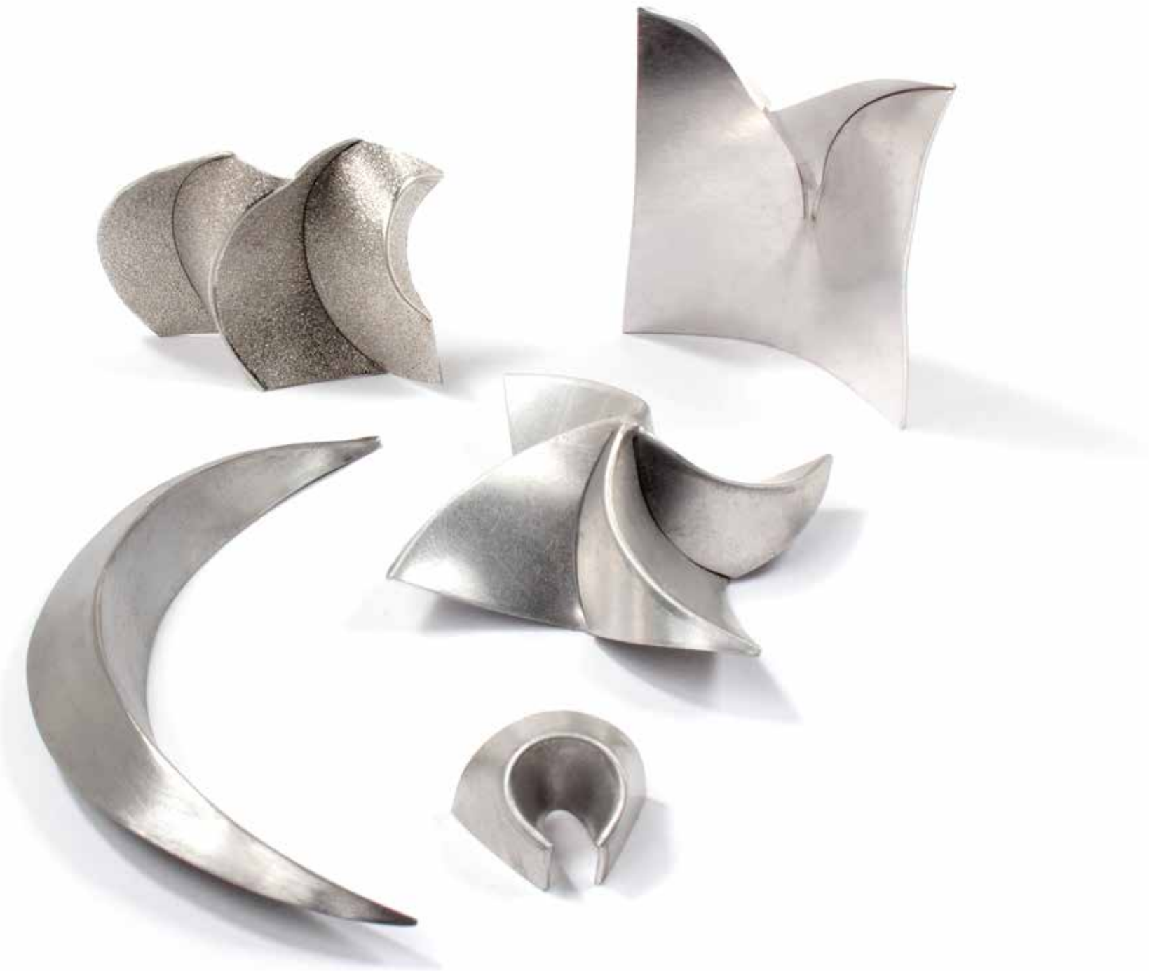
Samples of curved score folds made in aluminium, mild steel and pewter.
