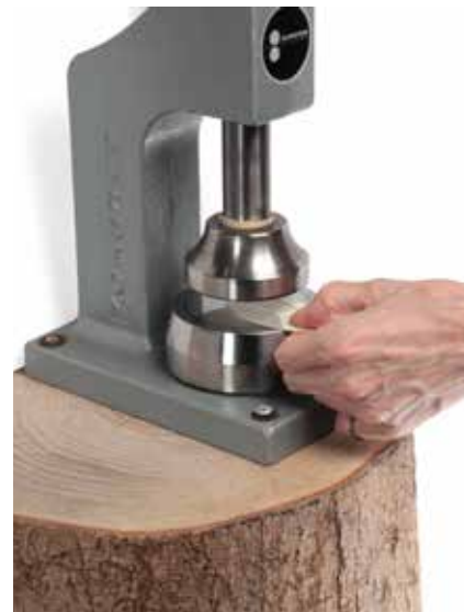
Using a Planishing Press
