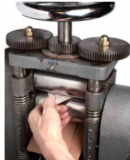
Scoring with a Rolling Mill
